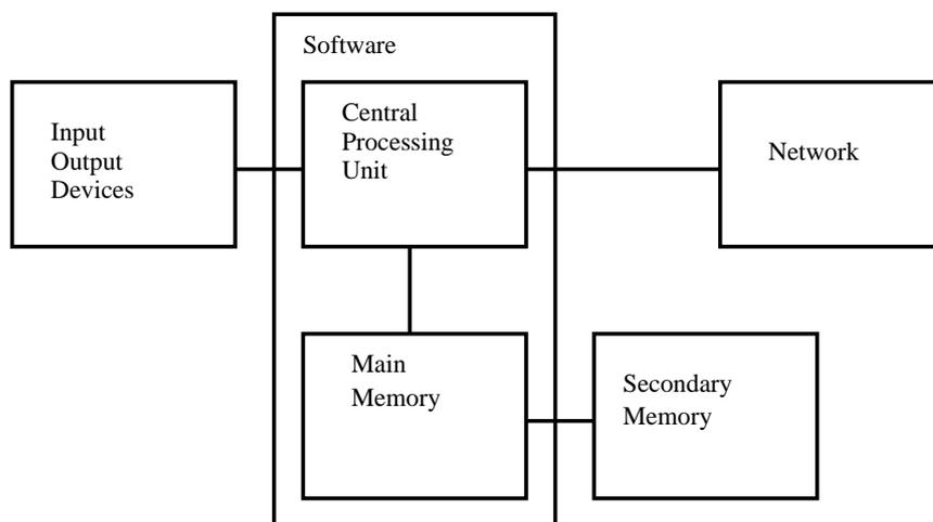
In this chapter, we start to work with **Secondary Memory** (or files). Secondary memory is not erased even when the power is turned off. Or in the case of a USB flash drive, the data we write from our programs can be removed from the system and transported to another system.
