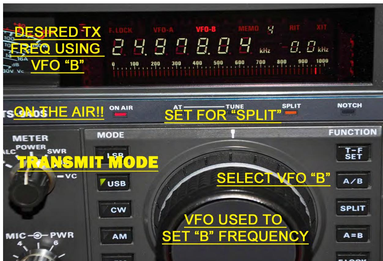
The most desirable set up, however, is to have what is called a “sub-receiver.” That gives you the capability to transmit on one frequency, to receive on that same frequency, and at the same time to receive on another frequency. We will talk more about a sub receiver’s advantages in a minute.
