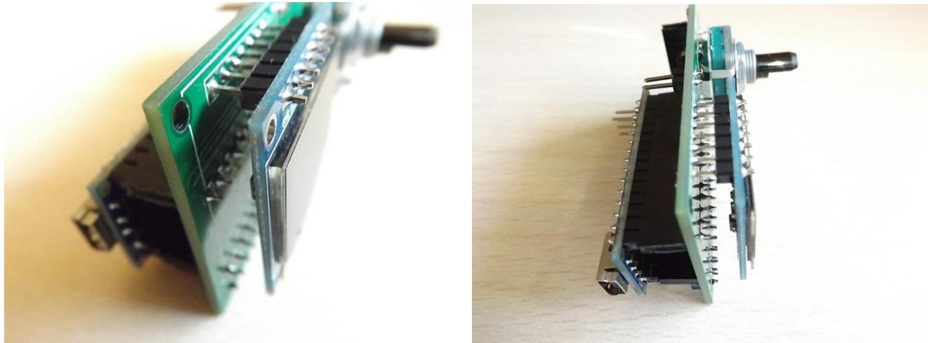
Note: When solder the strips of pins, make sure they are straight and flat on the board.
