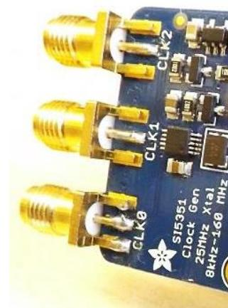
**IMPORTANT: The outputs are not decoupled DC. If the circuit where you are going to connect the signal does not include it, you must add a 10nF or 100nF capacitor in series with the signal.**
