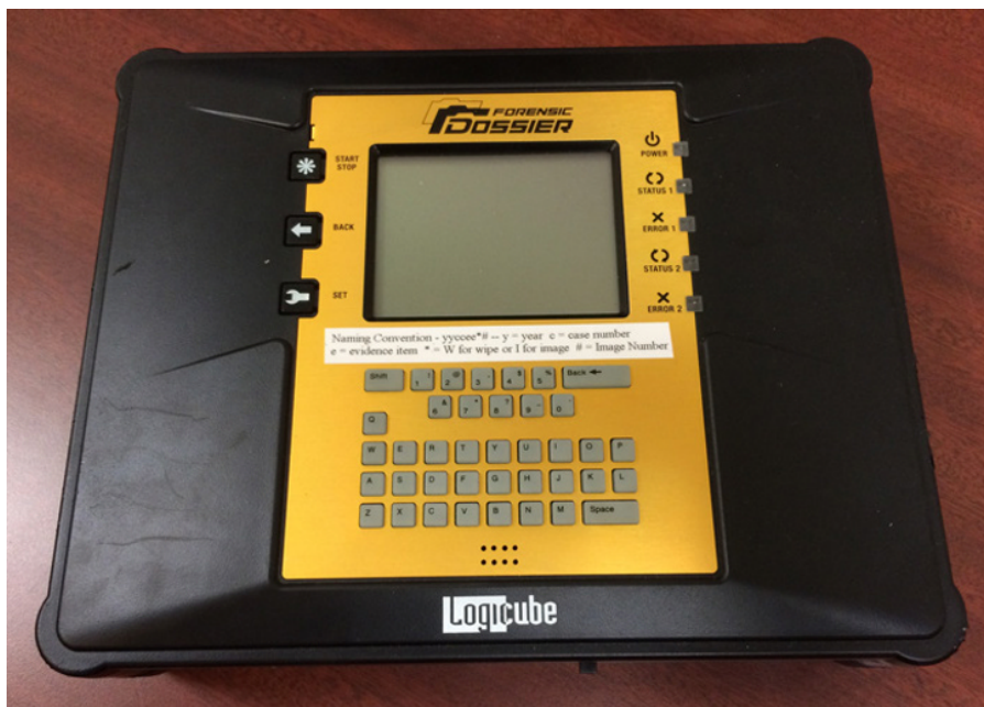
FIGURE 7.7 Logicube's Forensic Dossier duplicator device
