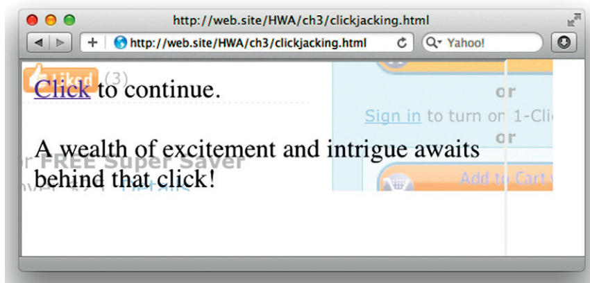
Figure 3.6 The overlay for a clickjacking attack
