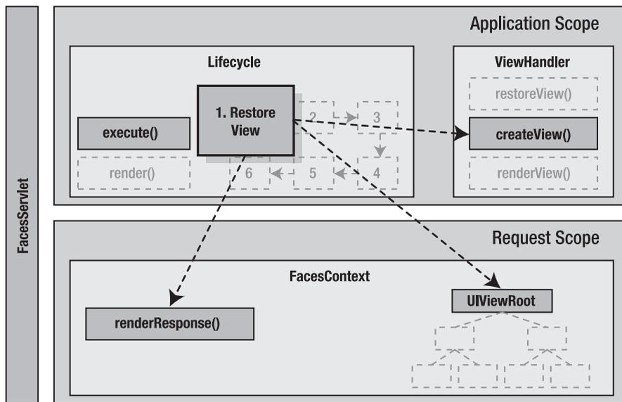
**Figure 1-11.** Restore View phase during initial request
