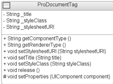
**Figure 8-12.** Class diagram showing the `ProDocumentTag` class
