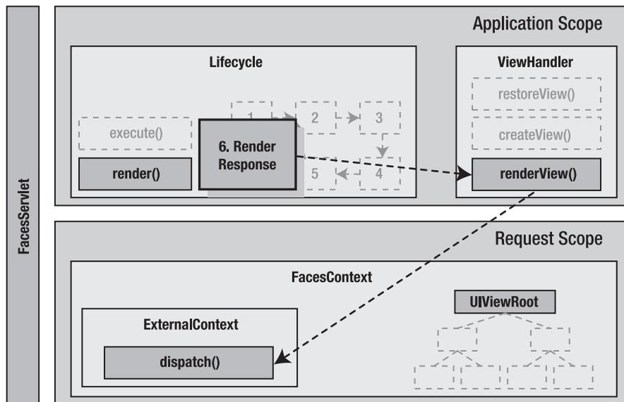
**Figure 1-12.** *Render Response phase during initial request*
