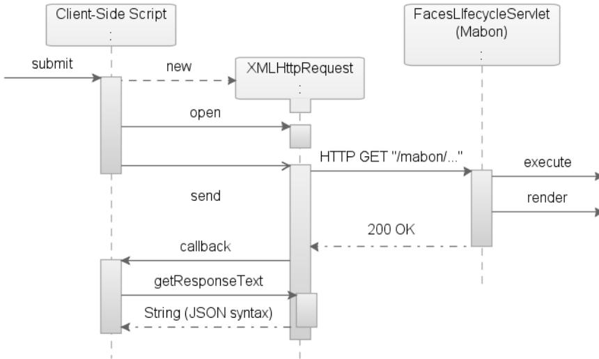
Figure 7-9. Sequence diagram of Mabon/Ajax data fetch request
