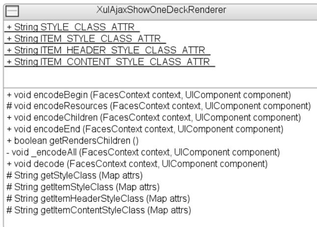
**Figure 8-10.** Class diagram showing the `XulAjaxShowOneDeckRenderer` class
