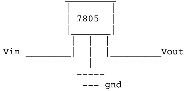
Vin = Voltage in, 6-12 volt wall adaptor, + goes to Vin, - goes to gnd
