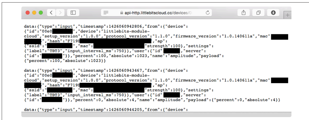
FIGURE 7-23. Gathering information about the connected cloudBit using the cloudBit API
