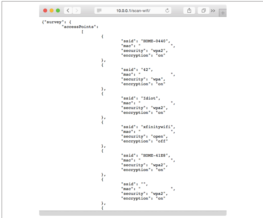
FIGURE 7-20. cloudBit query to obtain list of WiFi networks in range
