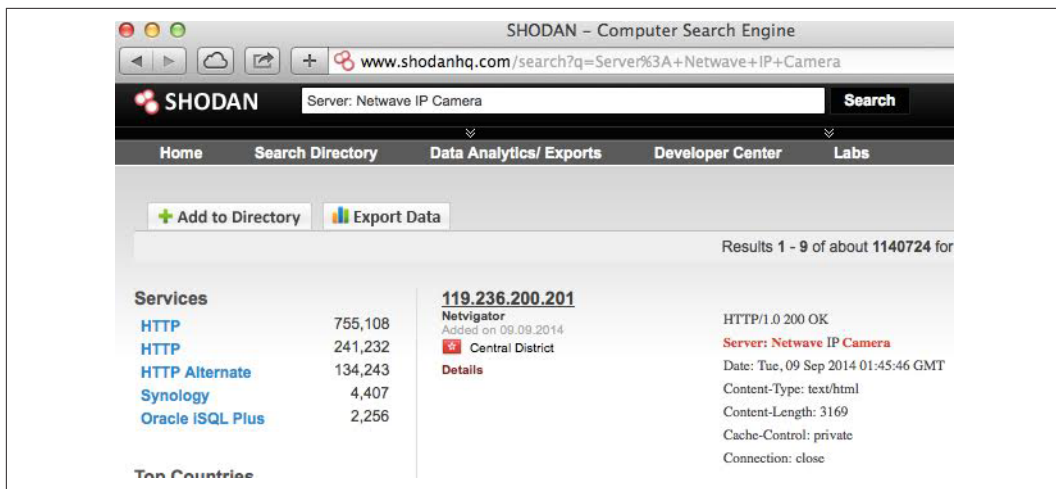
FIGURE 3-3. Shodan query to locate Foscam devices on the Internet
