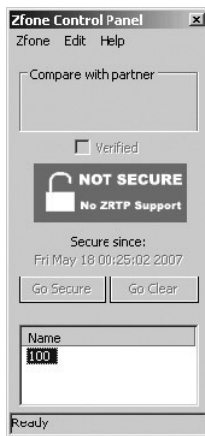
Figure 9-4: Zfone Not Secure usage with X-Lite soft phone
