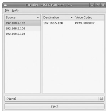
Figure 4-14: Injection audio with RTPInject
