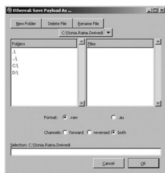
Figure 4-9: Saving RTP packets to an audio file
