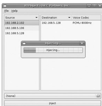
Figure 4-15: RTP injection audio replacement
