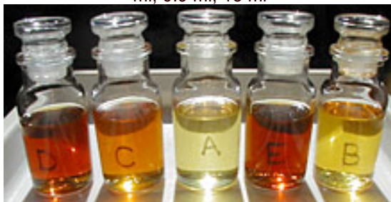
Best to worst by titration, left to right -- not what you'd expect just by looking. The longer oil is cooked and the higher the temperature, the poorer the quality will be, but the colour of used
