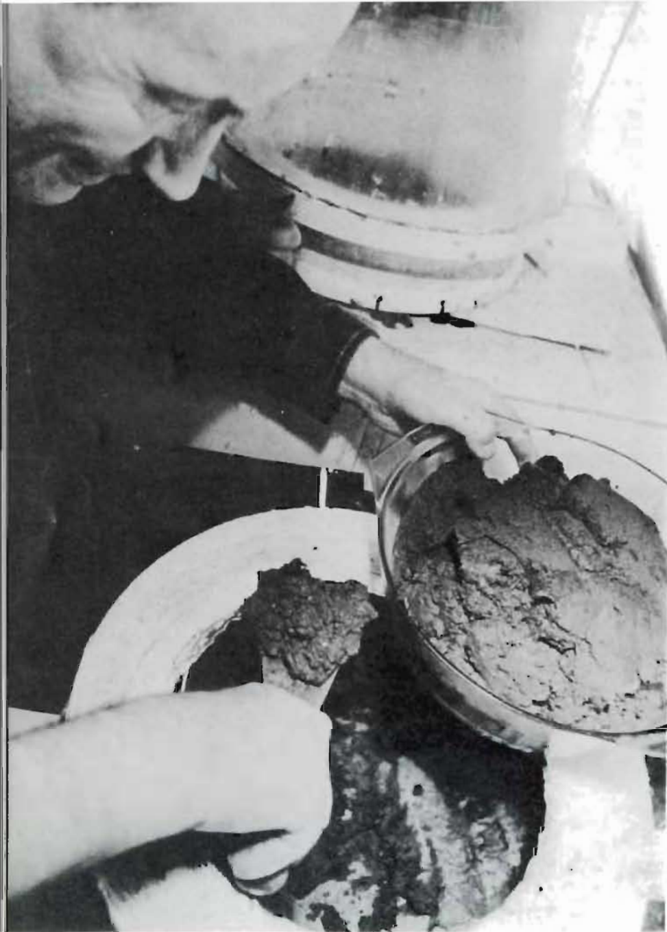
Regenerated peat. After several months' work heating and moistening the matter in the alambic one takes out a black substance which has assimilated
