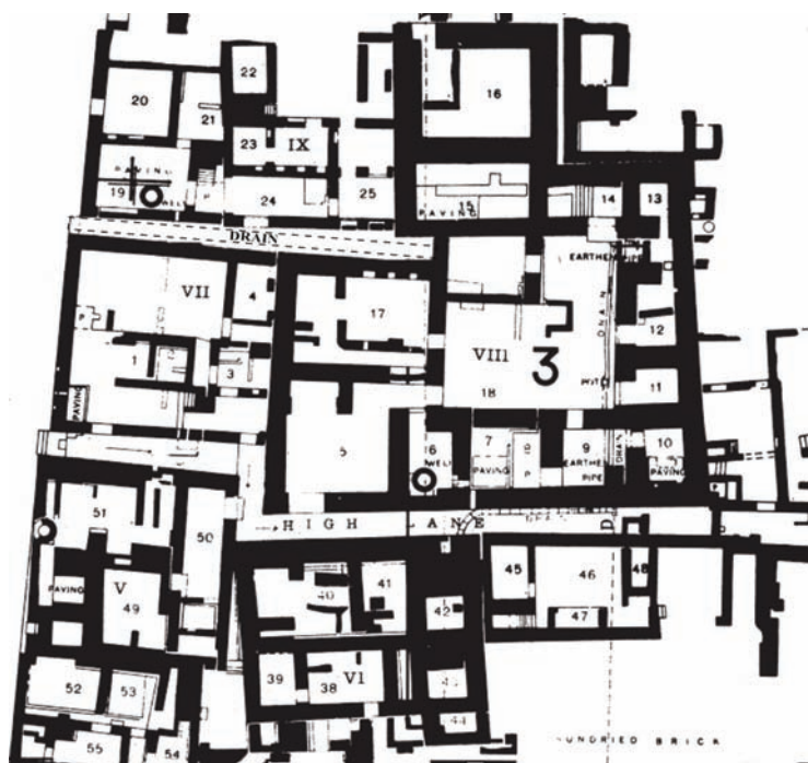
FIGURE 14.4. Plan of houses at HRA-B Mohenjo-daro. At top left, House VIII has a terracotta pipe (dashed lines) extending from its interior out to the main street. (Courtesy of M. Jansen, Aachen Research Project Mohenjo-daro)
