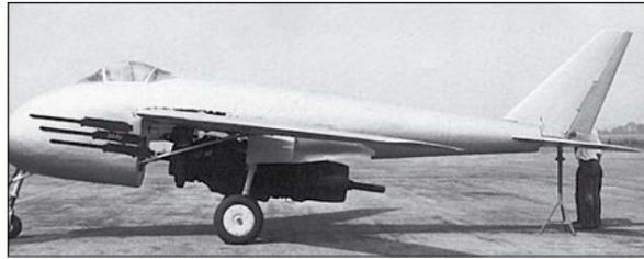
The P-1101 with engine and dummy cannon mounted (probably only after the war), but without engine casing, wing-fuselage transitions and rear fuselage section. (Photo: US Army)
