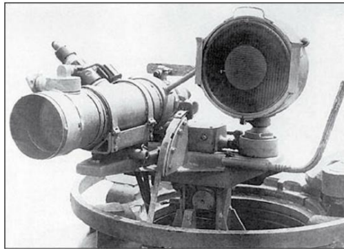
The FG 12/50 on the turret of the Panther tank . (Photo: CIOS)
