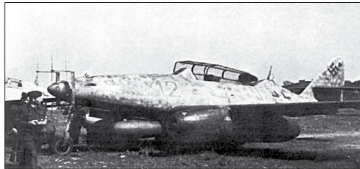
The Me-262V-1a/U1 – a two-seat night plane equipped with radar. (Photo: Military Archives)
