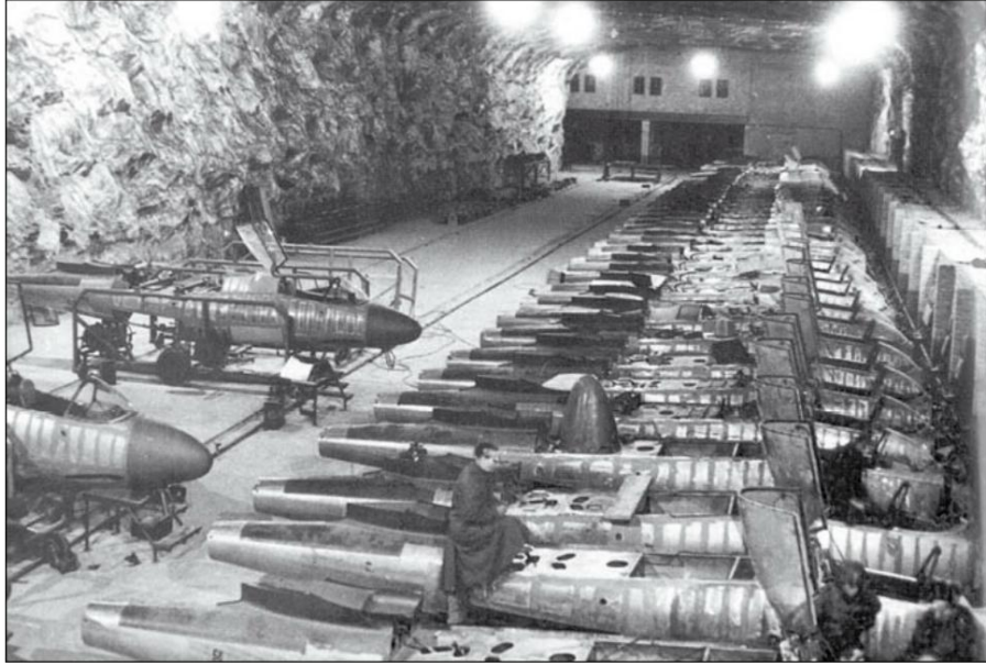
Unfinished He-162 fuselages in the gallery of an underground factory - probably "Tortoise"
