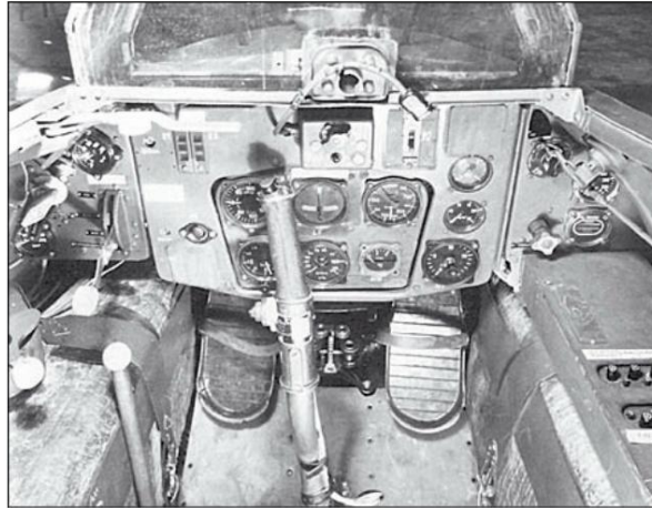
The shockingly simple cockpit of the Me-163. (Photo: NARA)
