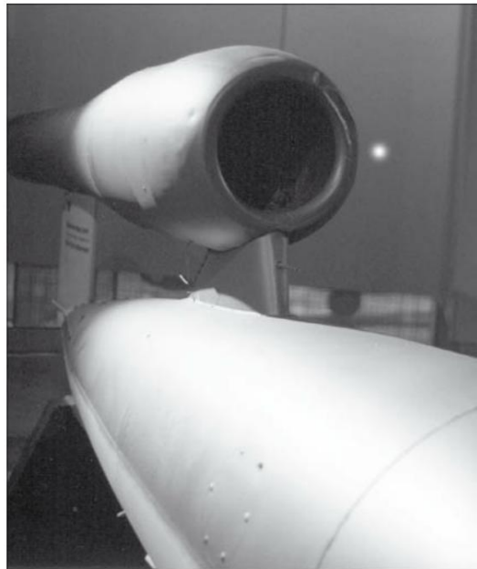
The V1, close-up of the air intake opening. (Photo: I. Witkowski)
