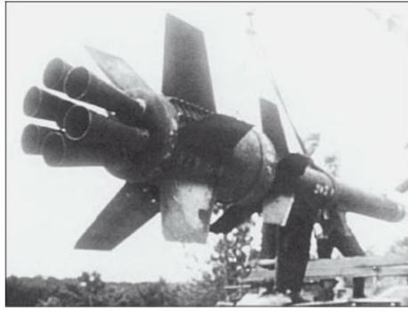
A close-up of the six nozzles of the Rheinbote rocket's main engine. (Photo: Imperial War Museum)
