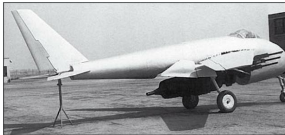
The P-1101 with engine and dummy cannon mounted (probably only after the war), but without engine casing, wing-fuselage transitions and rear fuselage section. (Photo: US Army)
