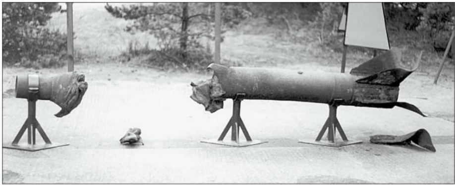
Parts of the Rheinbote rocket that exploded after launch near the test site in Leba. (Photo: I. Witkowski)
