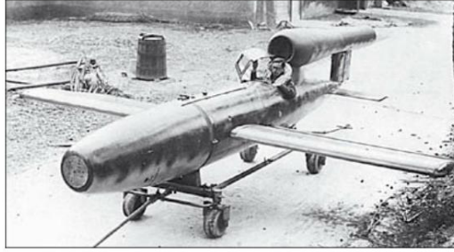
A suicide version of the V1 (the Fi-103 Re.4, without the nose section). (Photo: Imperial War Museum)
