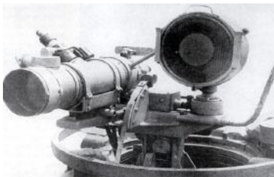
German Infrared Site Equipment Deployed on a PzKw. Panther Medium Tank 38
